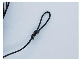
End loop on one of my (many) wire antennas for portable use. I attach my throwing line directly to the loop, foregoing an insulator. With smaller diameter wire, I sometimes put some shrink wrap over the GOOP.
